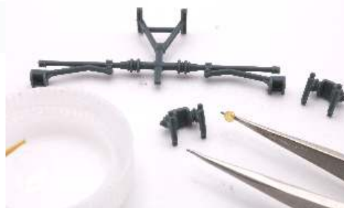
Use fine pointed metal tweezers to hold the magnet. Use a cocktail stick to apply a very small spot of glue into the cup in the Registration Arm or Catenary Wire Support
