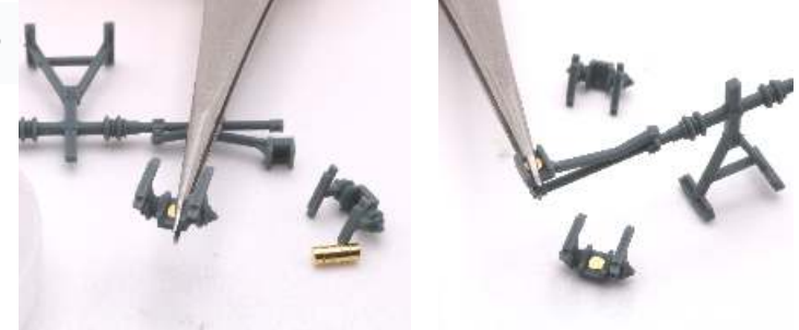
Carefully align the magnet with the cup and gently squeeze into place until the magnet is fully home
